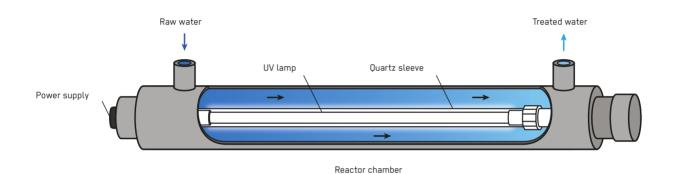
Under correct design and operational conditions, Ultraviolet (UV) Light can have anti-bacterial and anti-viral properties and can destroy pathogenic organisms in nonturbid water.
